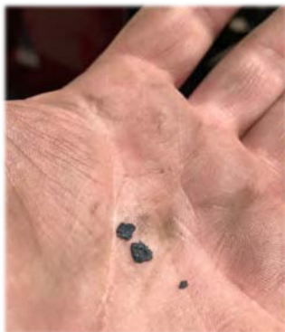
SLAG FROM HEAT EXCHANGER CASTINGS FOUND IN MANIFOLD
